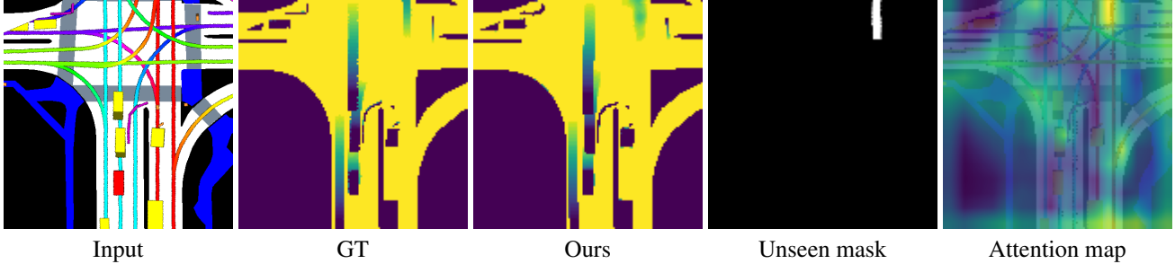
Figure 6. Visualization of attention masks W . For the attention map, the brighter area in the image indicates more significant responses. The attention map has higher responses around the unseen mask, thereby helping the model predict the motion of unseen vehicles.
